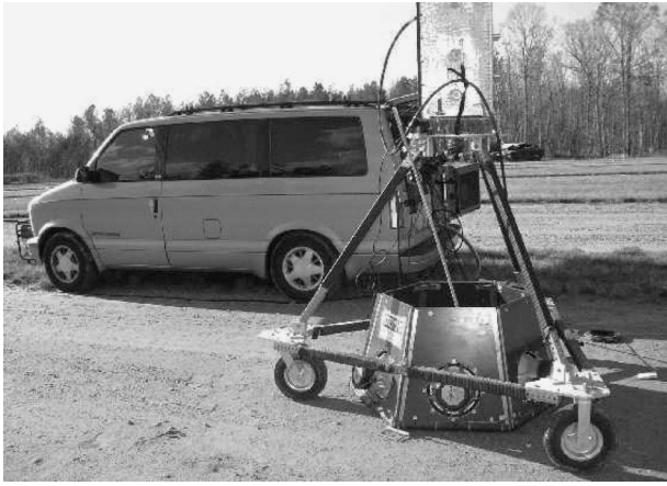
FIG. 9. An experimental setup for the seismo-acoustic landmine detection.
